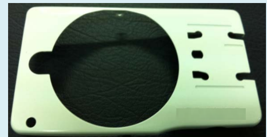
Coating of metal using the 2 coats, 2 bakes method
